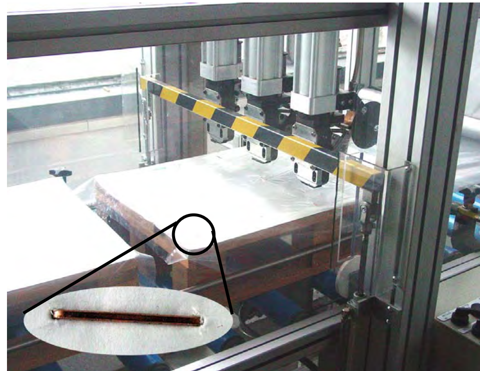
Nailing of foil and/or cardboard into wooden pallets
